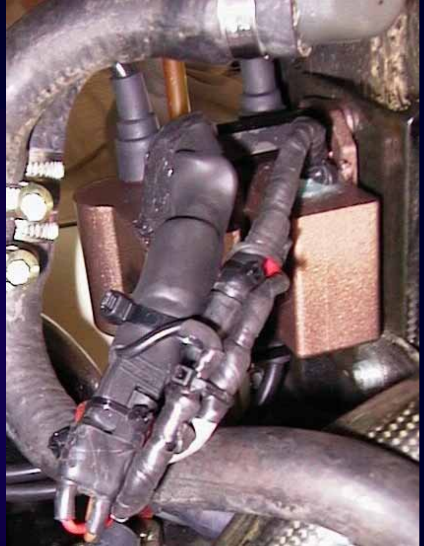
Modified by owner: no connectors and e- boxes at centerline of vibrations
