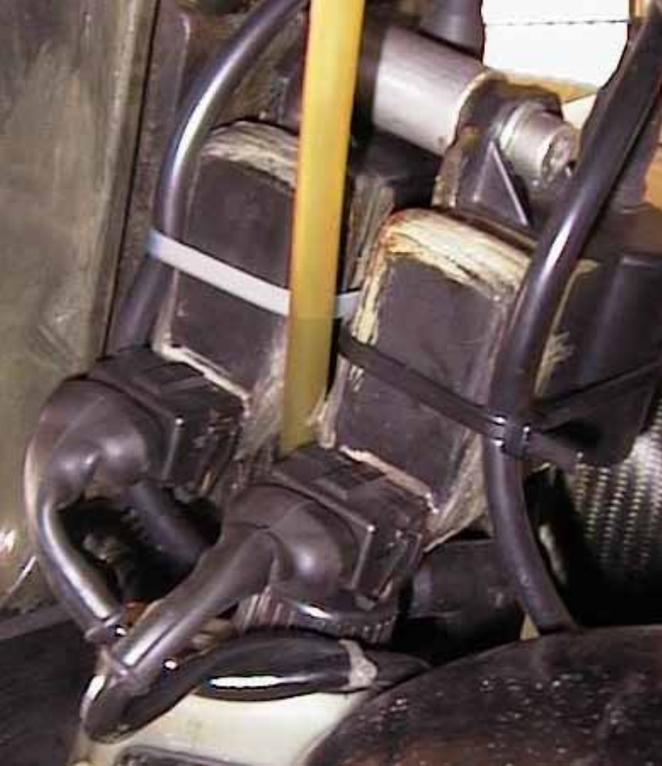
Modified by owner: original connectors and e-boxes at centerline of vibrations
